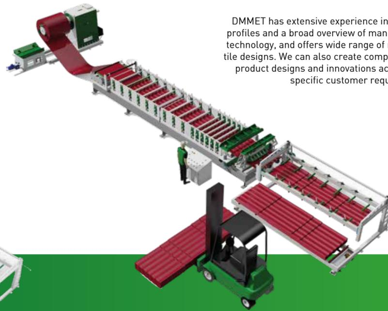
DMMET has extensive experience in metal tile profiles and a broad overview of manufacturing technology, and offers wide range of metal roof tile designs. We can also create completely new product designs and innovations according to specific customer requirements.
